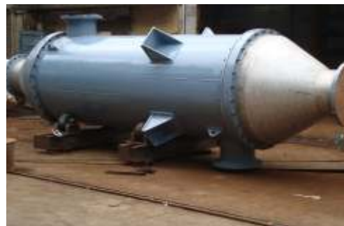
401 m 2 Economiser Client: Alok Industries
