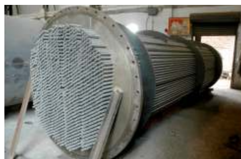
Tube Bundle assembly in progress of 309 m 2 Exported to Aditya Birla Chemicals (Thailand) Ltd.
